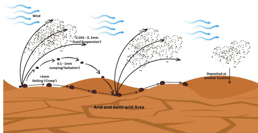
**Figure 1.** Different sizes of soil particles move due to wind at the transportation stage [21].
